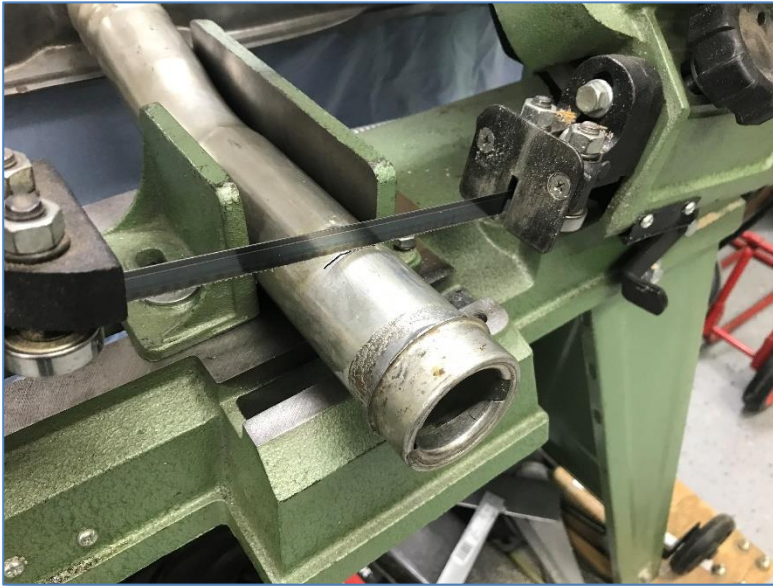
Figure 2: Cutting off the original filler neck end.
