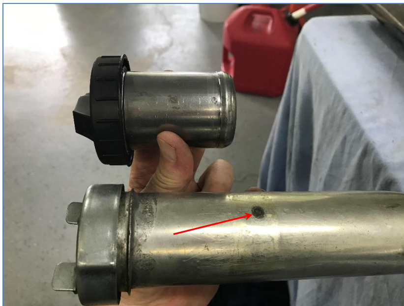
Figure 1: NJ-2-20-F Universal filler neck from Filler Neck Supply Co. and cap next to the stock filler neck.
