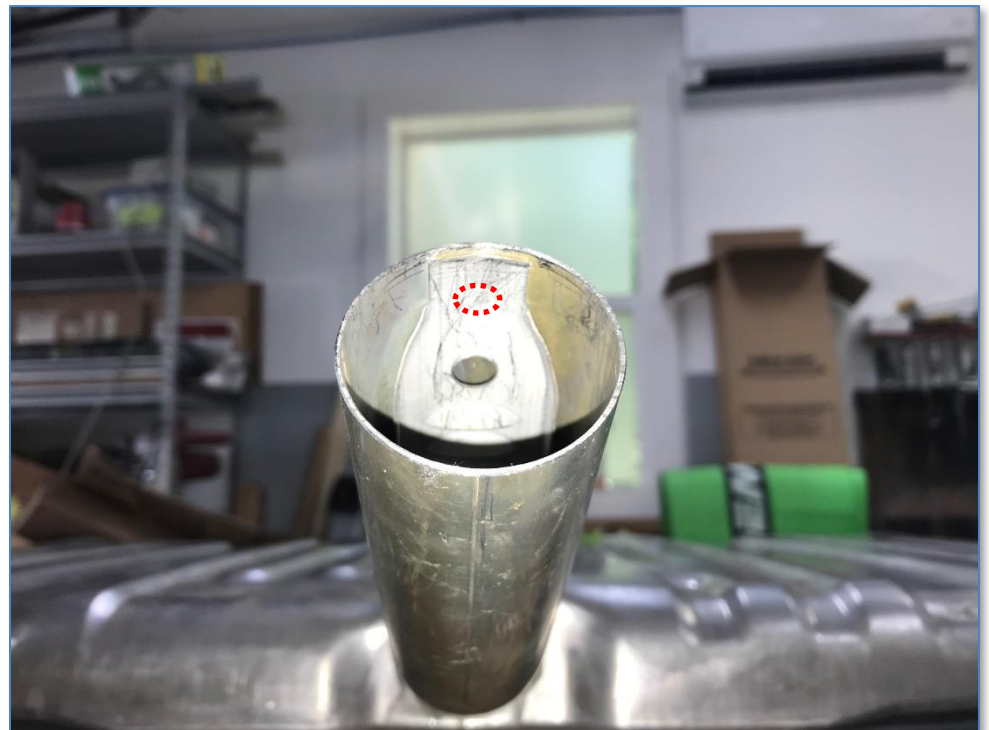
Figure 3: Filler neck after cutting, showing the end of the internal splash baffle. The spot-welded area is shown in red.
