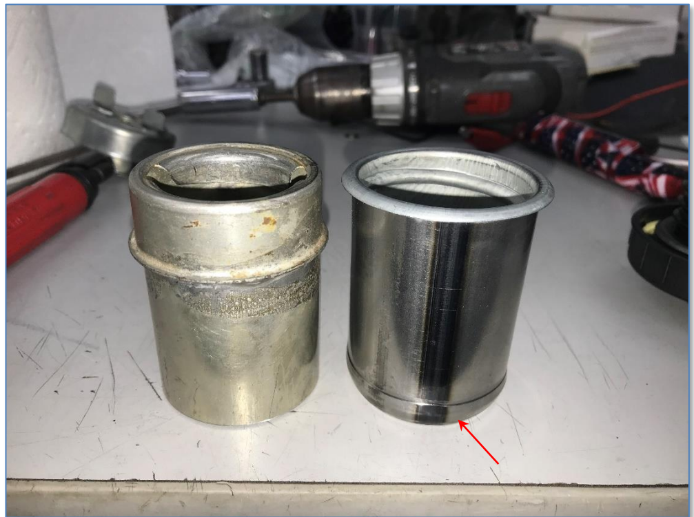
Figure 4: Cutt-off and replacement comparison. Ultimately, the barb end (arrow) of the replacement filler neck was also removed to facilitate a proper butt end connection.
