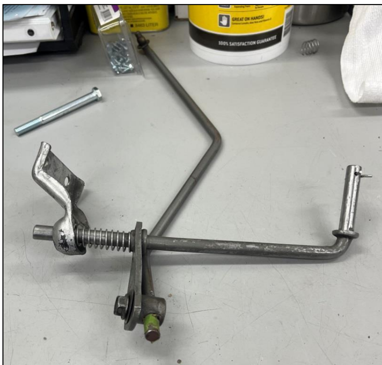
Photo 3: The Interlock linkage assembly removed from the vehicle.
