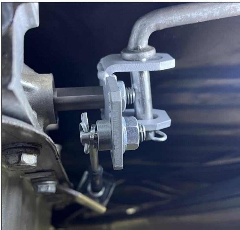
Photo 2: Correct bracket for the 4L60E but modified with "ears" from the old bracket
