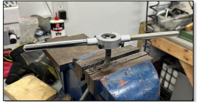
Photo 5: Threading the remaining stub end after the cut
