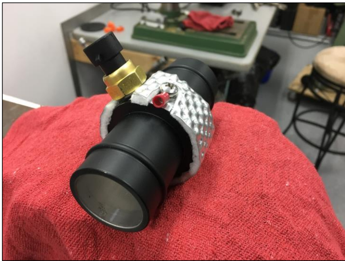
Photo 4: Assembled with insulation on exposed sections as a precaution against potential heat-soak. The connector is for a separate ground.
