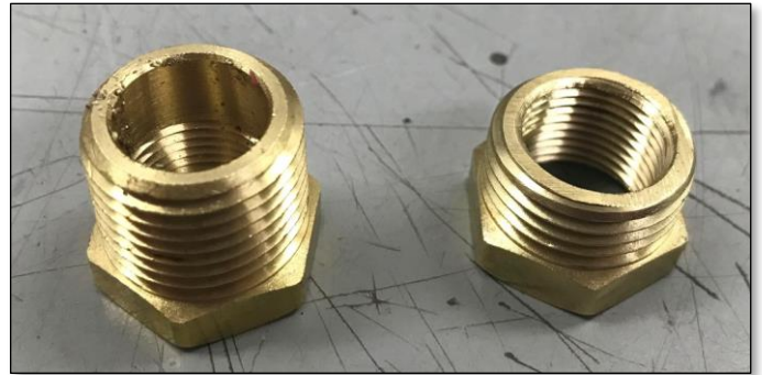
Photo 7: The modified intake manifold adapter: Before (L) and after (R).
