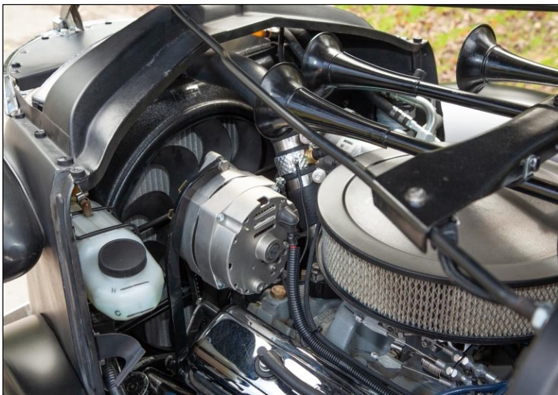
Photo 1: Swapping a small block Chevy V8 for the original 6-cylinder engine makes for a very cramped and hot engine bay.
