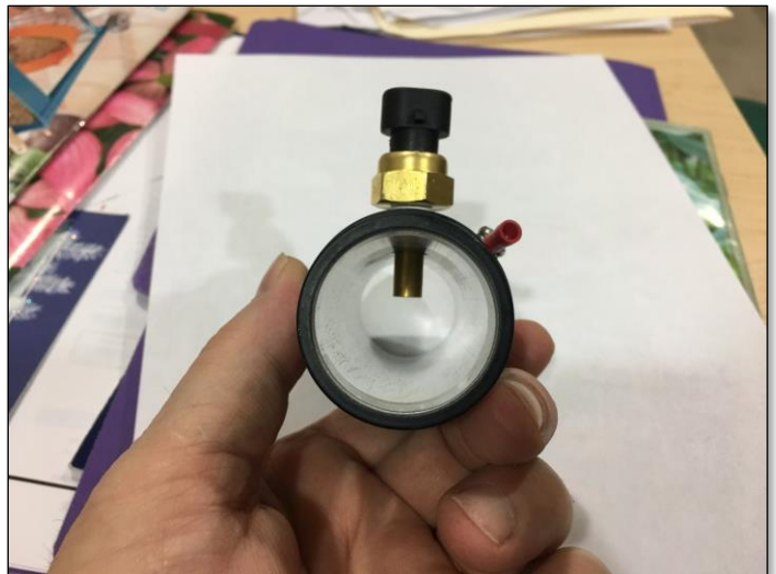
Photo 3: End view showing proper water flow probe placement.
