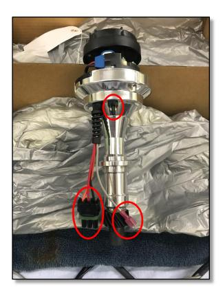
My distributor came highly polished. This seems to be the default. Instead of a vacuum advance mechanism, there is a small port on the underside of the body where you would attach your vacuum line. This vacuum line must be connected to full a manifold vacuum source and not a ported source.
