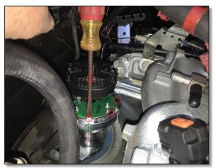
The inside lip of the distributor housing has eight black marks, indicating where the rotor would fire a plug wire – three are visible in this picture, circled in red. Go ahead and rotate the housing so that the rotor tip lines up with the nearest of the black marks as shown.
