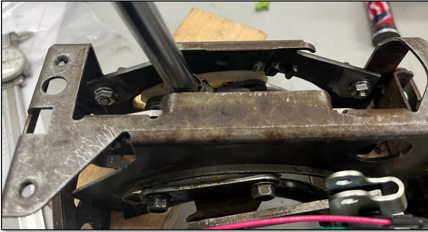
Photo 4: Modified stop plate reinstalled
